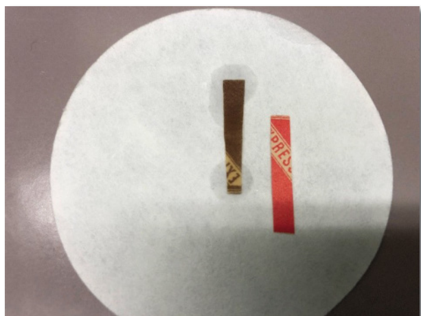
Fig. 6: Comparison of an Orient Express vignette discoloured brown by lead sulphide in the above experiment with an (original) red vignette.
